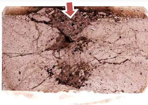
*Damage in UHPFRC under impact loading*
